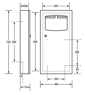
This product is AS1428.1 compliant (accessible compliant) when installed in accordance with the guidelines.
